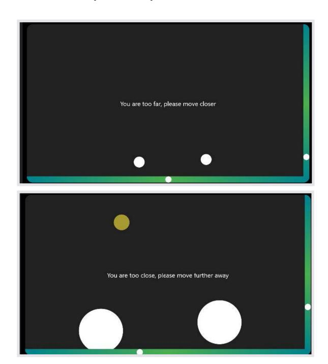
Calibration starts automatically as soon as a correct position is kept for a certain time.
