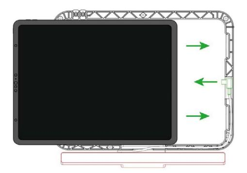
**3.** Place the front panel on the iPad. Make sure the clips snap into place, flip the case and apply the screws.
