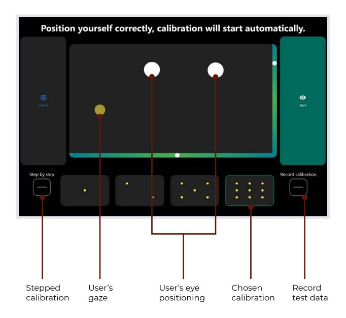
Before a calibration is started, it is possible to select how many points are to be used for the calibration. A higher number of points takes longer, but usually achieves more accurate results.
